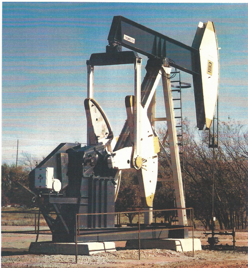
Two point mounting pads reduce installation cost.
