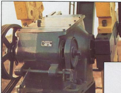
OIL IS WIPED OFF BULL GEAR AND FED INTO BACK SIDE OF BEARING FOR GUARANTEED OILING
