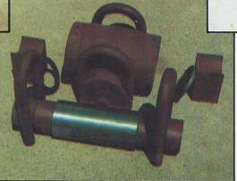
TAIL BEARING HAS 4" SHAFT WITH 9" BEARING SURFACE. 11/4" U BOLTS TO HOLD TO BEAM AND TO EQUALIZER. BRONZE BUSHINS.
