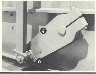
1 The construction is of fabricated steel for greatest strength and rigidity, as opposed to cast iron which is weaker and subject to breaking and cracking. 2 The chain reducer box is designed to be an integral part of the main frame to further increase the strength and rigidity of the unit. 3 All chains, sprockets and bearings are standard parts—readily available and easily field replaceable.
