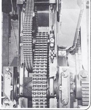
Wrist pins and Equalizer Bearings Wrist pins and pitman (equalizer) bearings are identical double spherical self-aligning roller bearings mounted in machined cast iron housings. Lubrication to these bearings can be accomplished from ground level.
