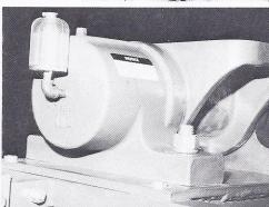
**Prime Mover** Cast iron "T" slot rails for mounting the prime mover clamp directly to the wide flange structure of the base, and adjusting screws are provided for belt tensioning.
