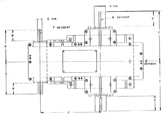
Shaft extension diameters listed are standard. Other diameters and keyseats can be supplied upon request.
