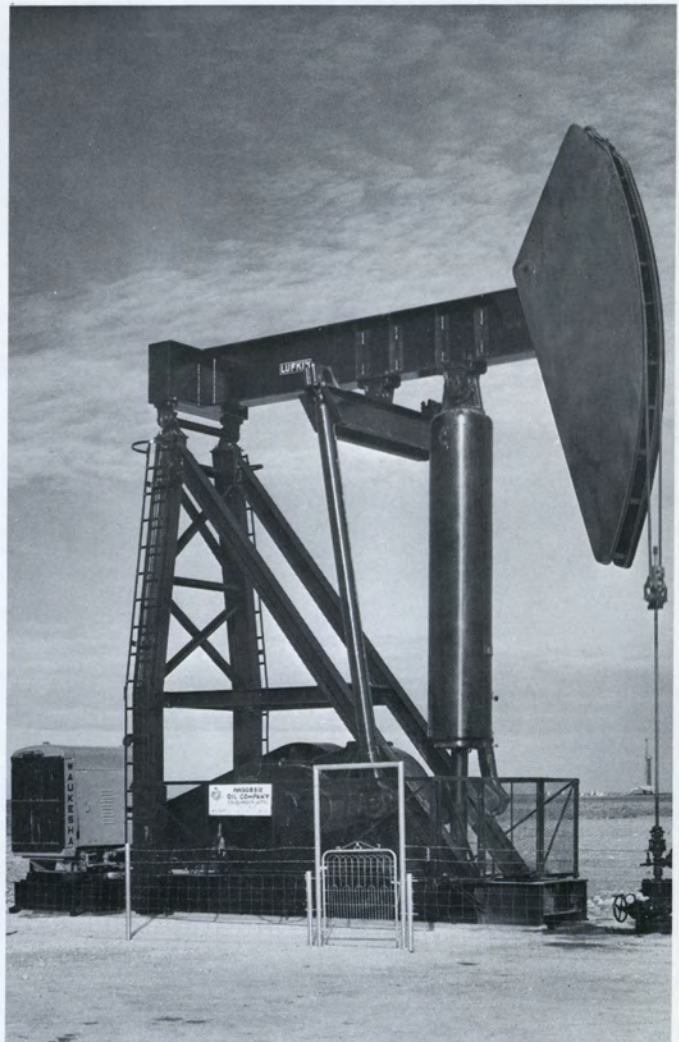
FIGURE 14 Lufkin A-1824D-192-42 Air Balanced Unit With Multi-Cylinder Engine Drive.
