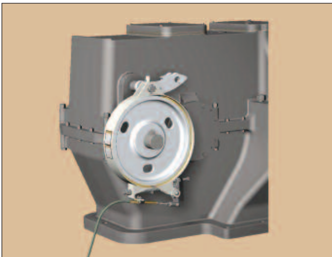
Flex-Shoe Brake. Provides much greater holding capacity than the Clam Shell type formerly used. Smoother acting with no "grabbing." Positive stop pawl can be engaged with notches in brake drum to provide additional safety. The pumping unit brake is not intended as a safety stop but is intended for operational stops only.
