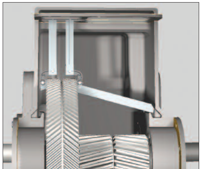
Consistent lubrication is essential even at low speed operation (below 5 SPM). This can be accomplished with the addition of optional high speed gear wipers for reducer sizes 912 and below. High speed gear wipers are standard equipment on reducer sizes 1280 and above.
