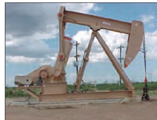
The Power Lift Unit design is conventional except for the addition of a "knee joint" in the rear Samson post leg which allows the post to fold, thus, lowering the beam and horsehead.
