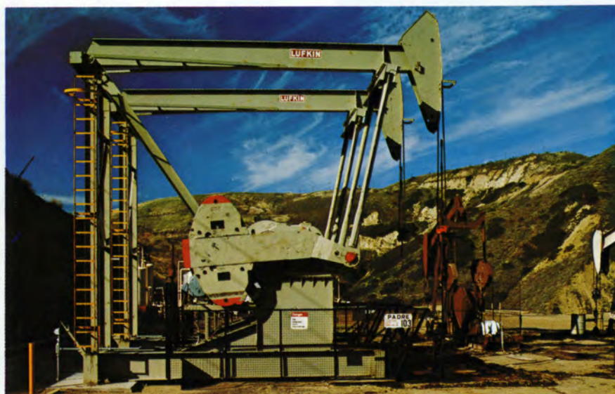
A pair of gas engine-drive M-320D-305-100 MARK IIs in Ventura, California. These units are capable of producing over 4,000 bf/d from shallow depths.
