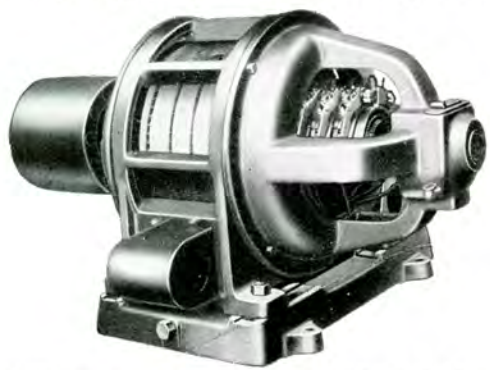
Type OMT-536, 35/15-hp., Two-speed Oil Well Motor, with Both Speeds Variable, for Pumping, Pulling, and Cleaning
