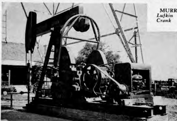
Figure 14 STROUBE & STROUBE, INC. Lufkin Double Reduction Twin Crank Unit—Waukesha engine drive.
