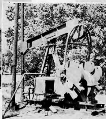
Figure 15 MURRAY & GOODE, INC. Lufkin Single Reduction Twin Crank with Waukesha engine drive.
