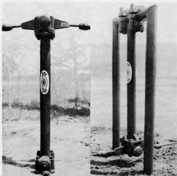
Figure 51 Lufkin hold-up and hold-downs. All bearings interchangeable and Alemite lubricated.
