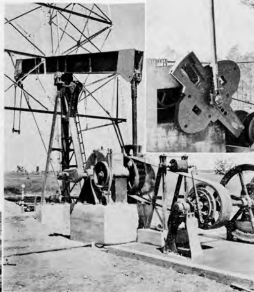
SINCLAIR OIL & REFINING CO. Lufkin 5½" Herringbone Unit with Lufkin Hoist and sand reel—electric motor drive.
