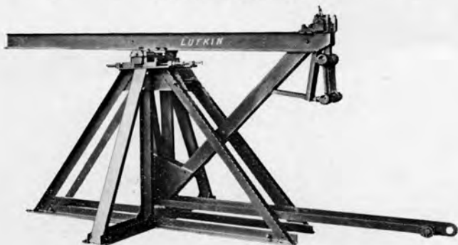
Figure 52 Lufkin underpull pumping jack. Electrically welded construction throughout—well braced and equipped with bronze bearings.
