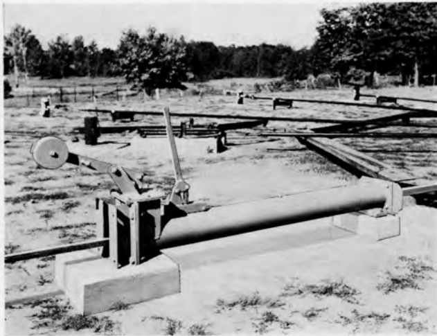
Figure 50 Trout patented Safety Coupler—a very simple, yet effective, mechanical device for hooking on and off from power—self-contained and designed for life time service.
