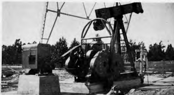
WEAVER-CRIM OIL CO. Lufkin single reduction twin crank unit driven by Chrysler gas engine. Figure 12
