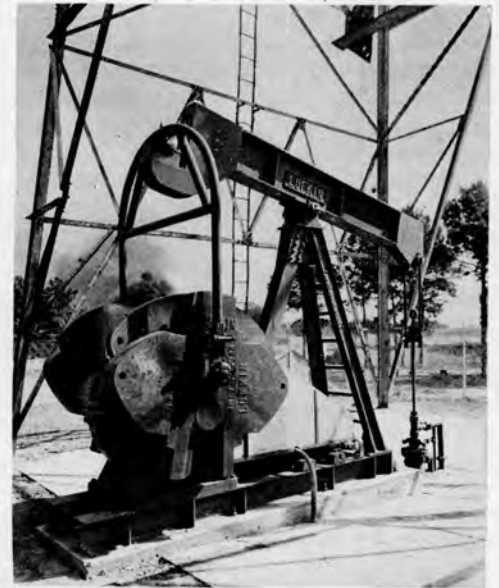
Figure 16 TIDE WATER OIL COMPANY Lufkin Single Reduction Twin Crank Unit— G.E. electric motor drive.
