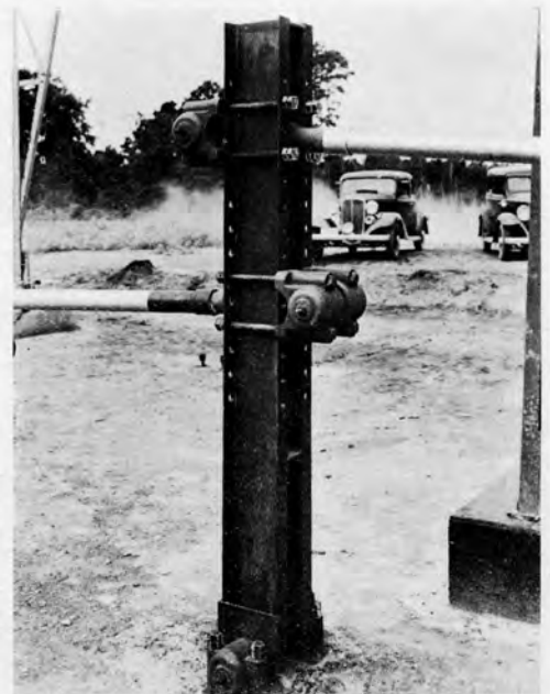
Figure 55 Lufkin stroke or multiplier post. This type also furnished with bearing in center position. Bearings on this post are interchangeable with hold-up and hold-downs.
