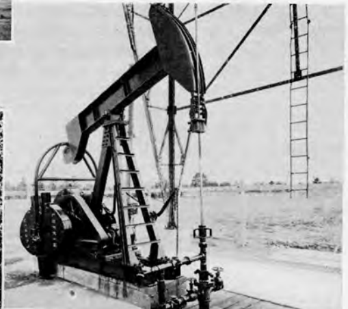
Figure 17 HUMBLE OIL & REFINING CO. Lufkin Single Reduction Twin Crank Unit— G.E. electric motor drive.
