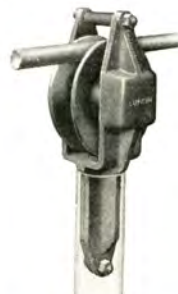
FIGURE 75 Lufkin Pull Rod Carrier; split malleable iron housing, 5" diameter gray iron sheave, paraffin maple bearings.
