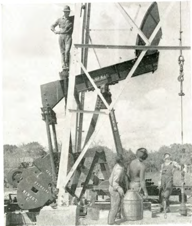
FIGURE 25—Showing hinged horse-head turned back over beam for servicing well
