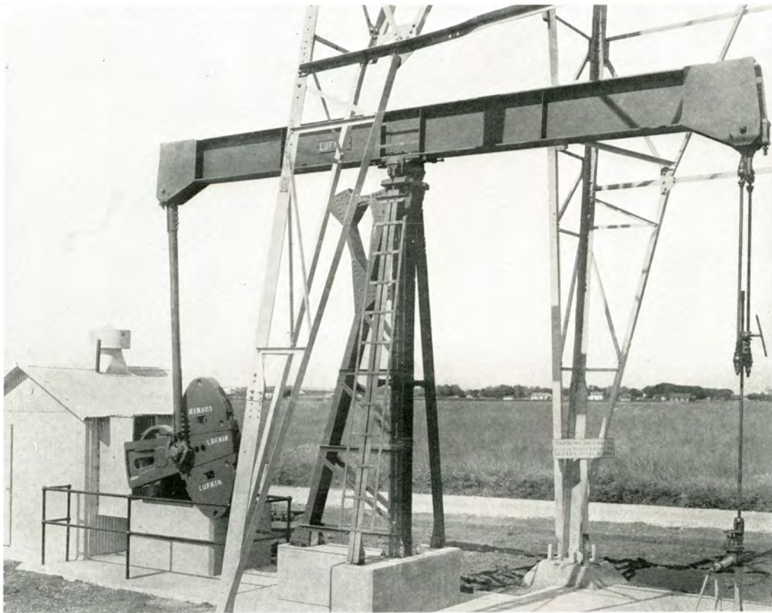
FIGURE 40—An East Texas installation Lufkin Single Crank Unit
