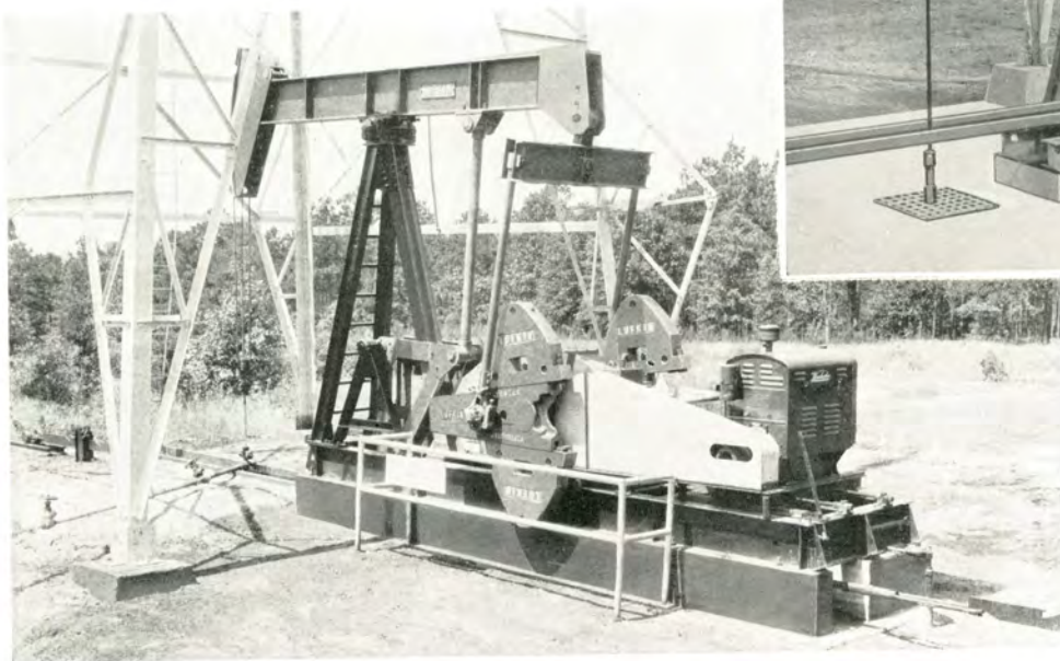
Lufkin Twin Crank Unit pulling two additional wells on an East Texas well under proration.
