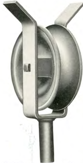
FIGURE 117—Lufkin 10" supporting sheave for 2½" pipe, commonly used with back crank take-off. The shank is made for 2" pipe and the sheave has a paraffined maple bushing.
