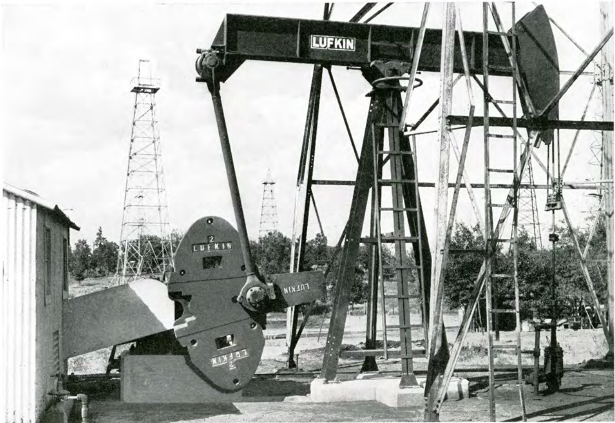
Top: Single Crank Installation—A-Frame Post, Safety Ladder, Universal Beam, with Hinged Horsehead, driven by multi-cylinder engine. Typical East Texas installation where Back Cranking is desired.
