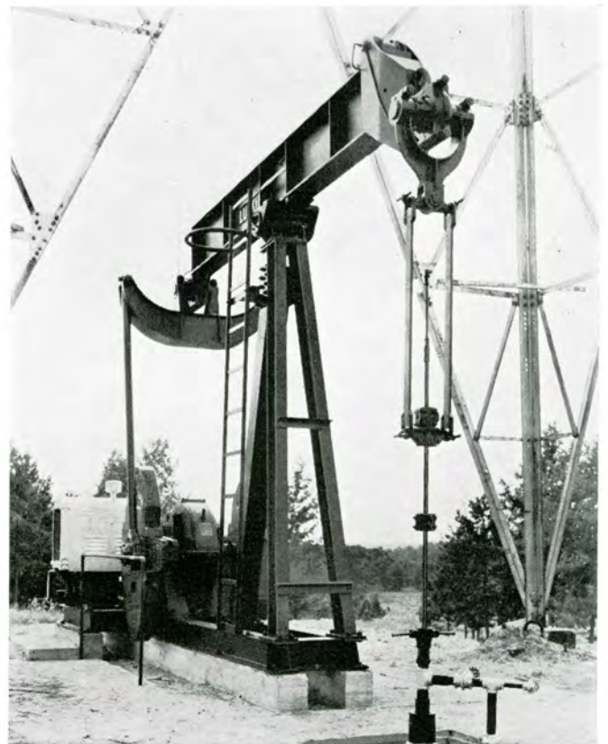
Below: New Unit No. 3A 16' Beam 8' Work- ing Centers, High Post, Hanger Head, Either No. 18A or 22C Gears.
