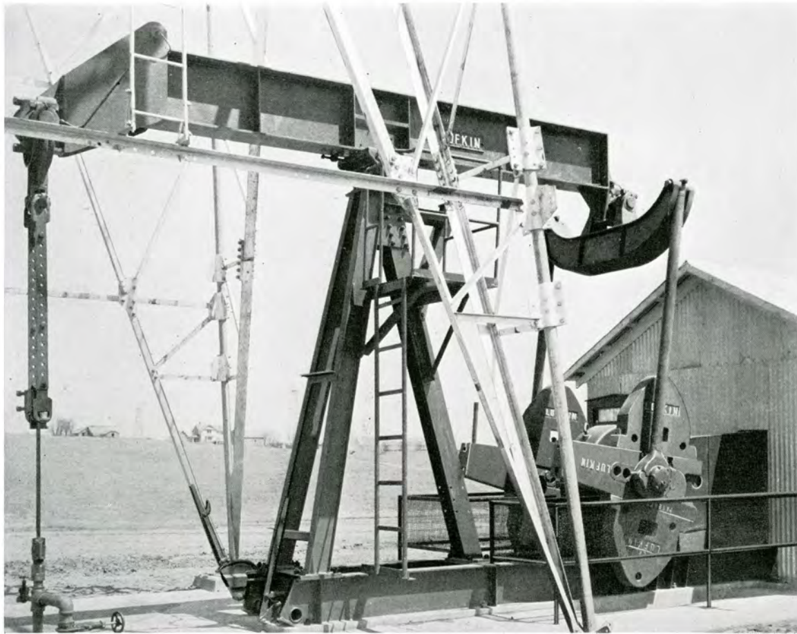
At left: T. C. 2A—54 Unit with 1020C Beam Single Cylinder En- gine Drive—Claf- lin, Kansas—with special platform for oiling beam bearings.
