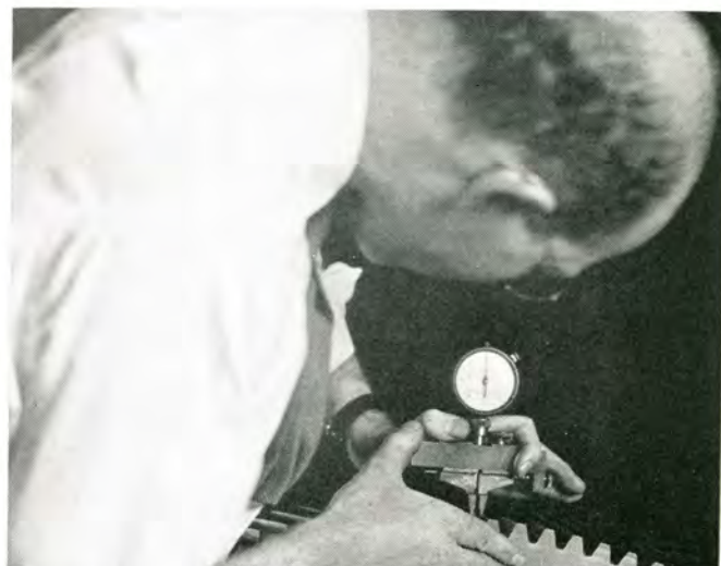
Teeth of herringbone gears must pass rigid inspection for accuracy of formation.
