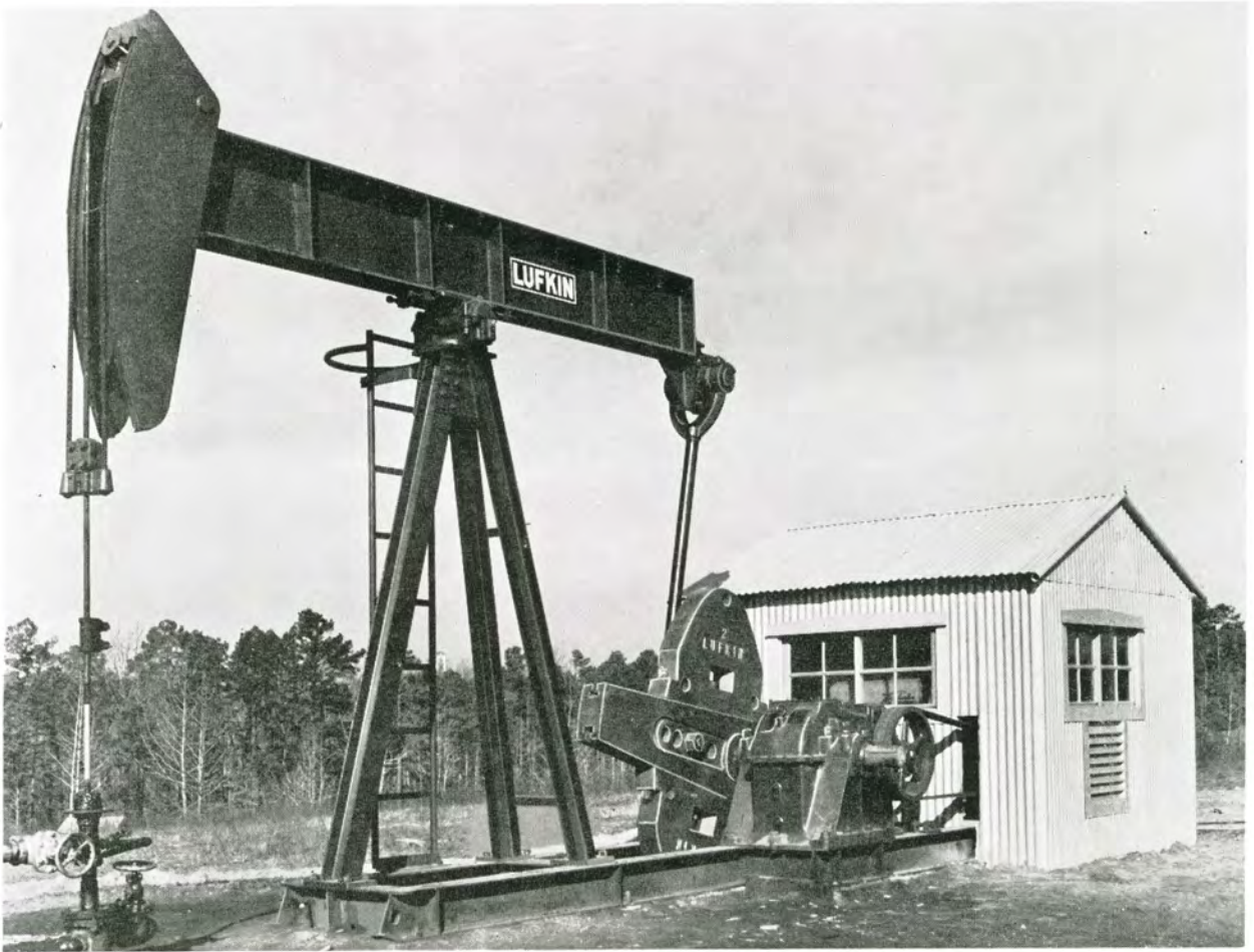
Single Crank Unit on Steel Base
