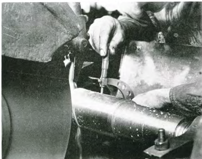
Grinding for accuracy. All shafts, pinions, crank pins, etc., are ground to absolute micrometer size.
