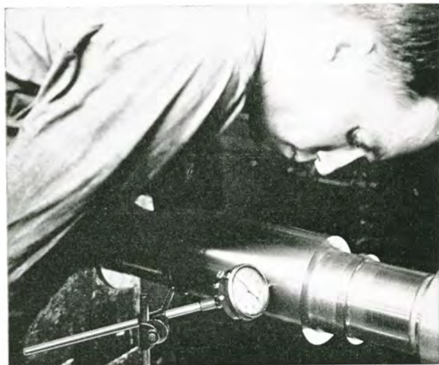
Testing pinion shaft blank for eccentricity before cutting herringbone teeth. Accuracy here is of extreme importance.
