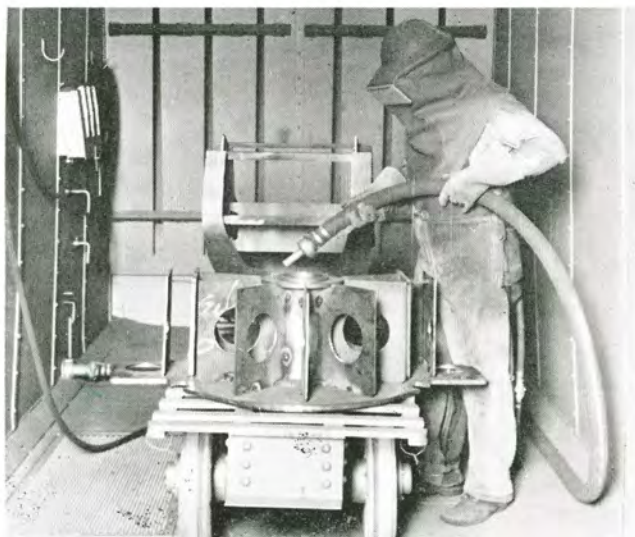
Casting and machine parts are sand blasted with modern equipment.
