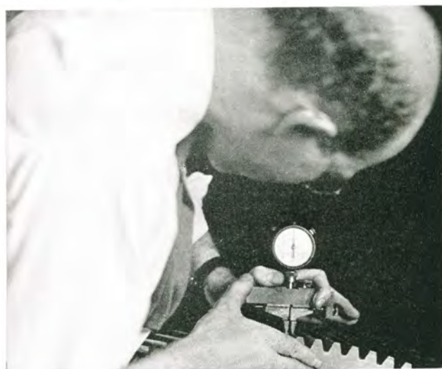
Teeth of herringbone gears must pass rigid inspection for accuracy of formation.
