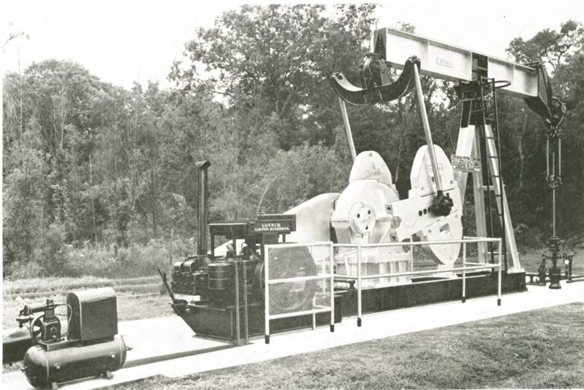
LUFKIN TC-2A-36A Twin Crank Pumping Unit with Sub base to clear sweep of cranks, bolted extension base to accommodate Lufkin Cooper-Bessemer GSDH 2 Cylinder Horizontal Gas Engine mounted on "T" Slots with pusher screws for tightening V-Belts, centerline type polished rod beam hanger.
