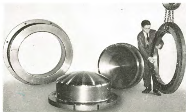
FIGURE 66 Die castings made of special alloy for presses up to 5000 tons capacity.
