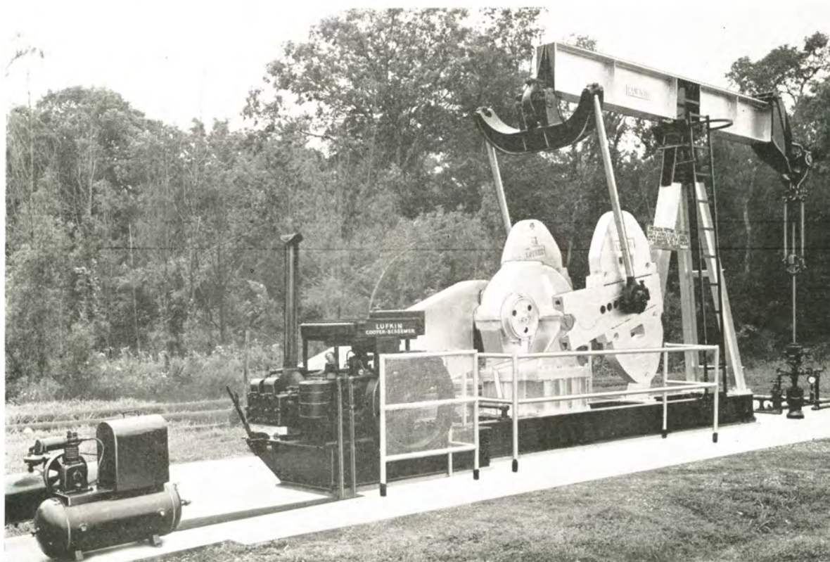
LUFKIN TC-2AT-36B Twin Crank Pumping Unit with Sub base to clear sweep of cranks, bolted extension base to accommodate Lufkin Cooper-Bessemer GSDH 2 Cylinder Horizontal Gas Engine mounted on "T" Slots with pusher screws for tightening V-Belts, centerline type polished rod beam hanger.
