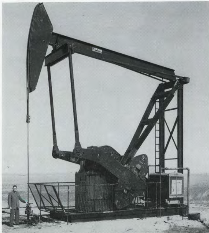
A Lufkin M-456D-253-144 Mark II Unit operating near Sterling, Colorado. Note compactness of drive when multi-cylinder engine is mounted within the samson post.
