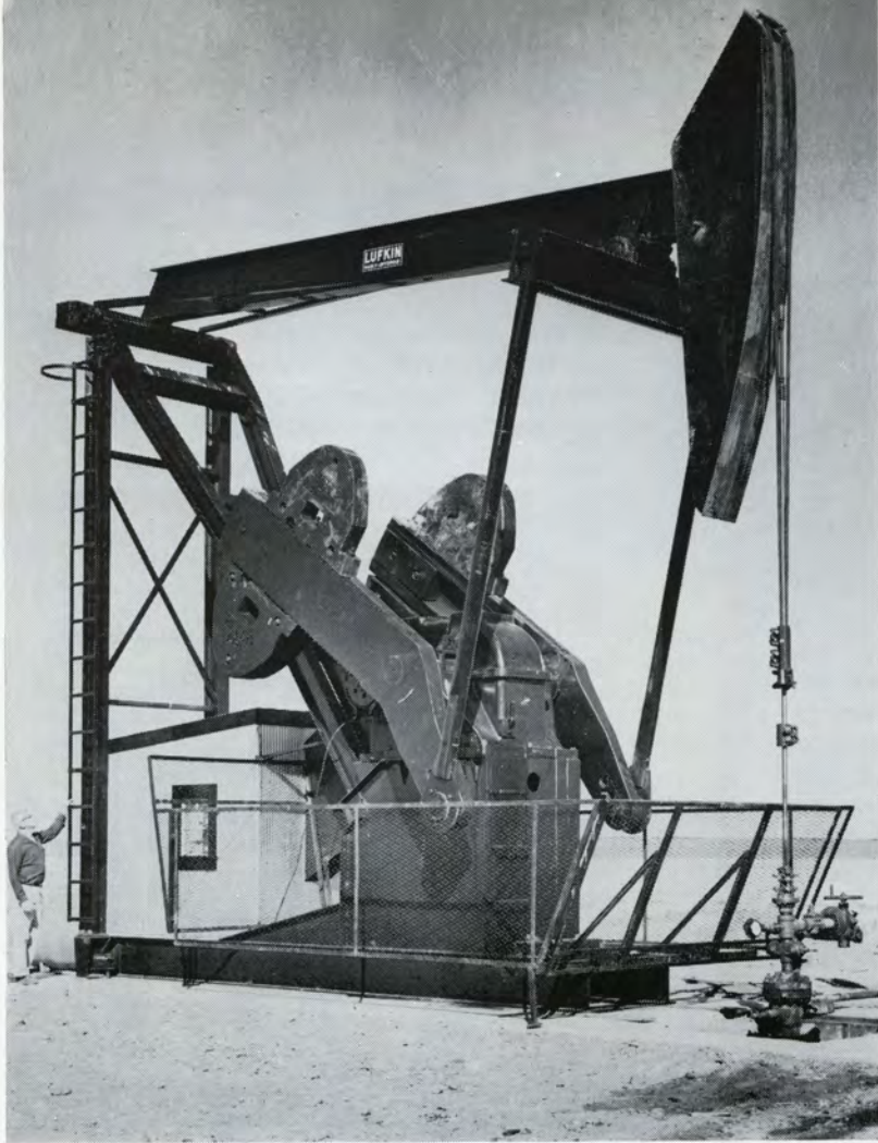
A Lufkin M-456D-253-144 Mark II unit with engine house for slow speed engine, pumping in Northern Montana.
