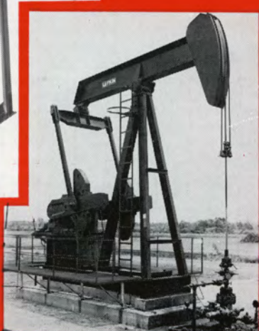
CONVENTIONAL PUMPING UNITS
