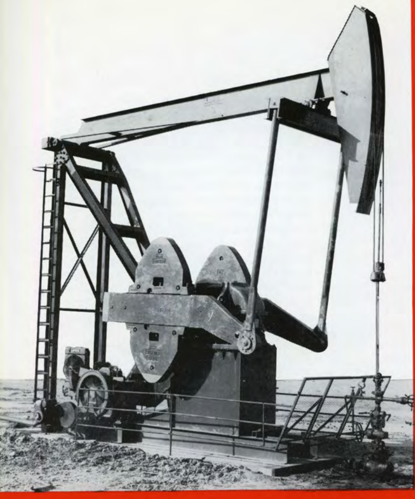
An M-640D-304-144 Lufkin Mark II, pumping in Southeastern Mississippi. The unit is driven by an H-795 Lufkin engine, counter-clockwise rotation, compactly mounted under the post on the main base sills.
