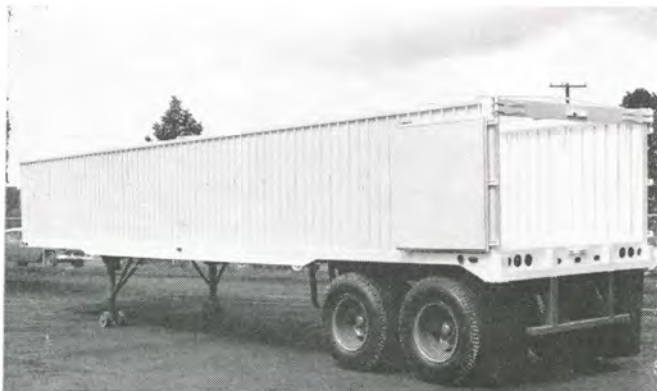
FIGURE 62 Model TOVLA Open Top Van (Light Weight) Steel for hauling all types farm & industrial products.
