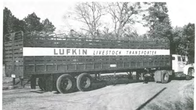
FIGURE 63 Model TOLS Adaptable for any type livestock haul (with or without roof).
