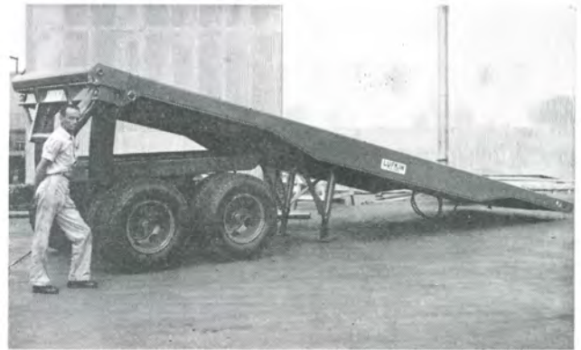
FIGURE 65 Model TOF-C A combination Float & Pipe Trailer (float can be easily attached or detached. TOF-50C can be used for pipe or machinery hauls).
