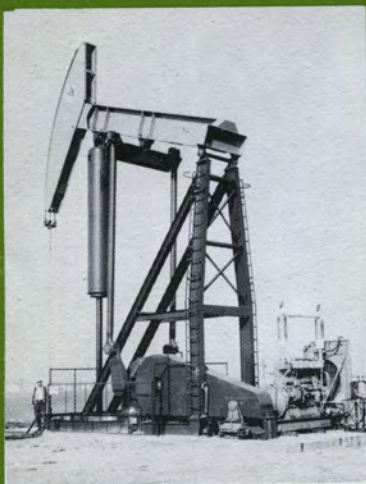
AIR BALANCE PUMPING UNITS
