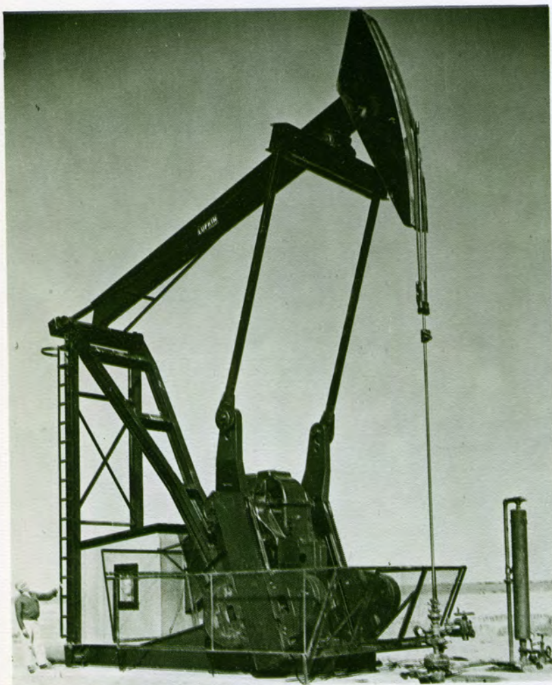
A Lufkin M-456D-253-144 Mark II unit with engine house for slow speed engine, pumping in Northern Montana.
