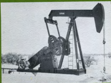
CONVENTIONAL PUMPING UNITS
