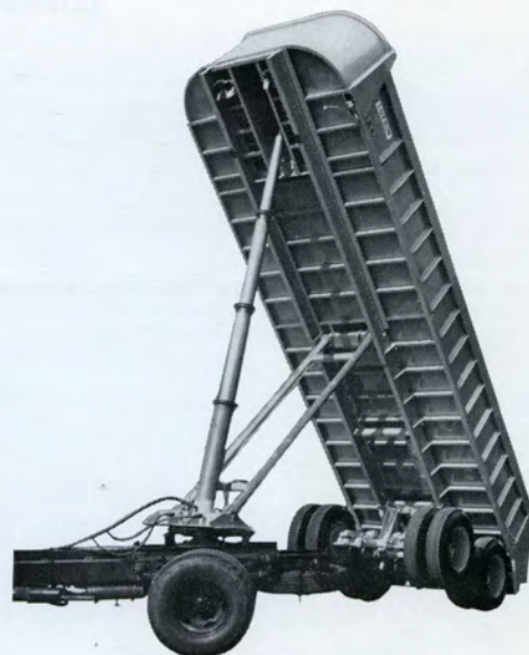
FIGURE 58 Model THD-2—Lufkin's Hydraulic Tandem Dump Trailer.
