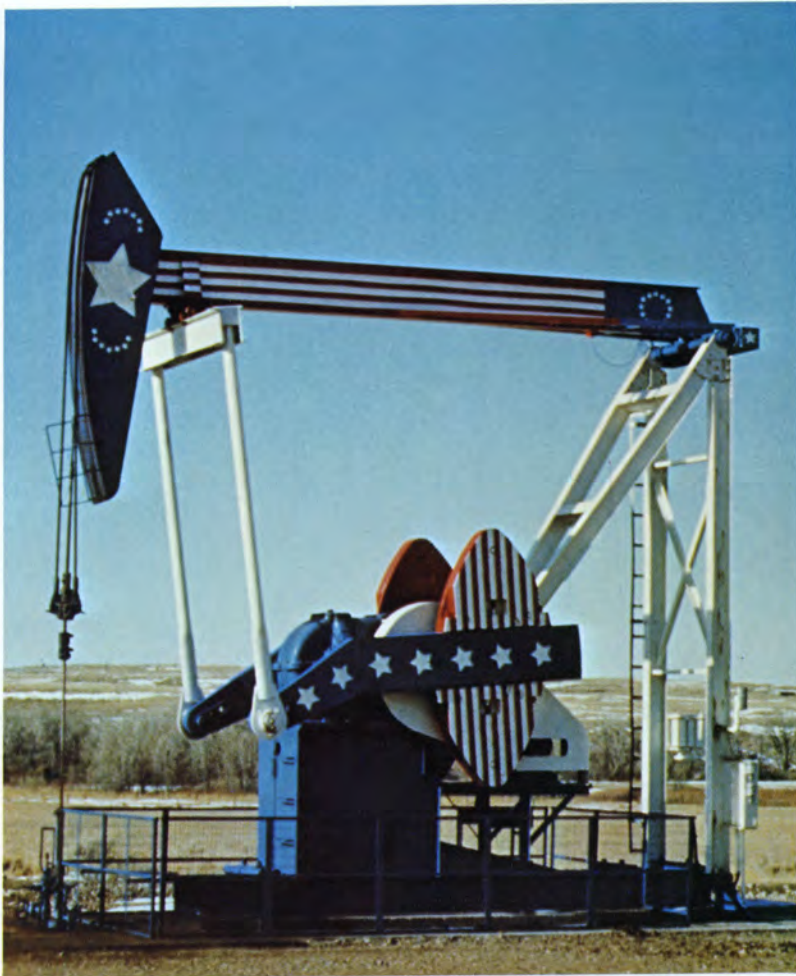
A Lufkin Mark II Unit dressed up for the Bicentennial celebration. A Mark II similar to this one (M-320D-256-144) produces 4000 BF/D from a water supply well in North Central Texas. Initially the unit pumped between 4000 and 5000 BF/D (reported maximum 5860 BF/D with a 5 3/4" casing pump)
