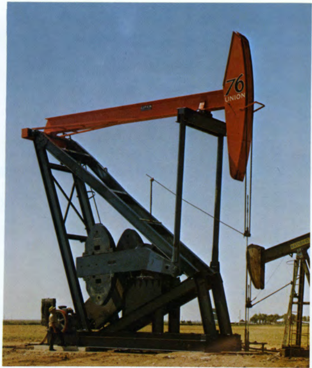
An M-1280D-427-216 Lufkin Mark II pumping 1050 BOPD from almost 8,000 feet with 2 1/4 inch pump at Farnsworth Unit Well 15-3.
