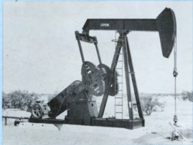
● CONVENTIONAL PUMPING UNITS
