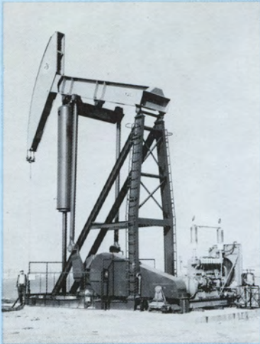
● AIR BALANCE PUMPING UNITS
