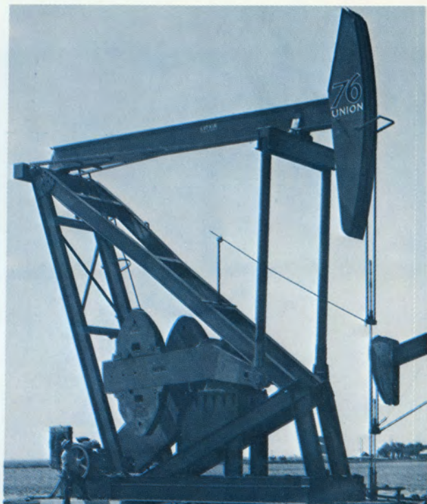
A Lufkin Mark II 1280,216 inch stroke, pumping 1050 BOPD from almost 8,000 feet with 2 1/4 inch pump at Farnsworth Unit Well 15-3.
