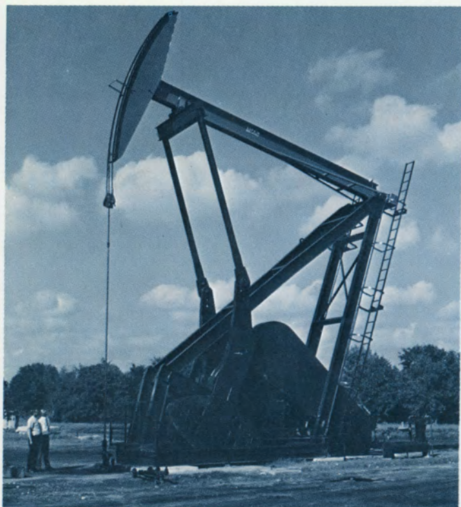
An M-1280D-427-216 Lufkin Mark II pumping unit lifting 1100 BPD from 5,600 feet near Woodward, Oklahoma.
