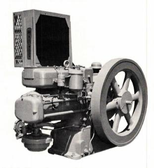
Lubrication of all working parts is assured by a combination splash and pressure system. Crankshaft main bearings, gears, governor and cylinder liner are splash lubricated. Connecting rod bearing is lubricated by a splash system and by-pass filter system.
