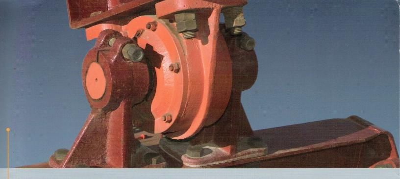
**Equalizer beam bearing assembly:** Unmatched in the industry for strength and durability, the assembly features machined ductile iron castings, oversized double row, self aligning roller bearing, metal to metal seals and large lubrication reservoirs. Sentry's design ensures constant equalization of loads to the pitman arms and crank pins. Proven, easy to maintain and extremely reliable in the long term.
