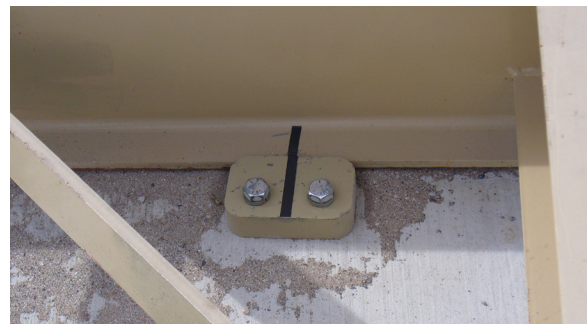
Alignment marking ensures proper positioning when the Rotaflex unit is moved to the operating or rolled-back position.
