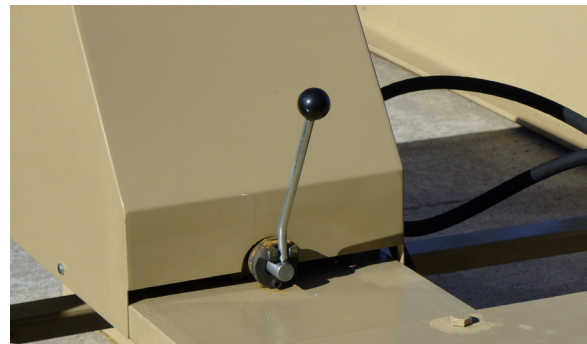
Operations stop when lever is released to ensure crew safety.
