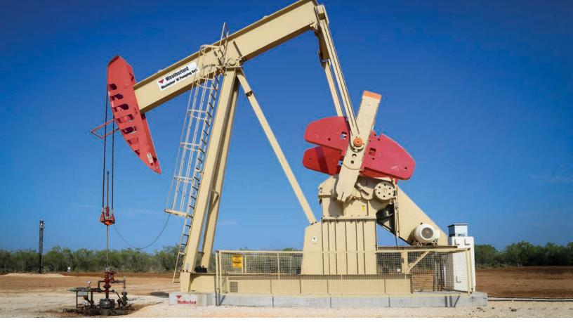
An optimized RRL system consists of a surface pumping unit powered by an electric or gas prime mover, a rod string, a positive displacement pump, a controller, and software.
